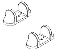
② Place the UPS in the stand. Always place with the left side of the UPS on the bottom, and the control panel on the top.
